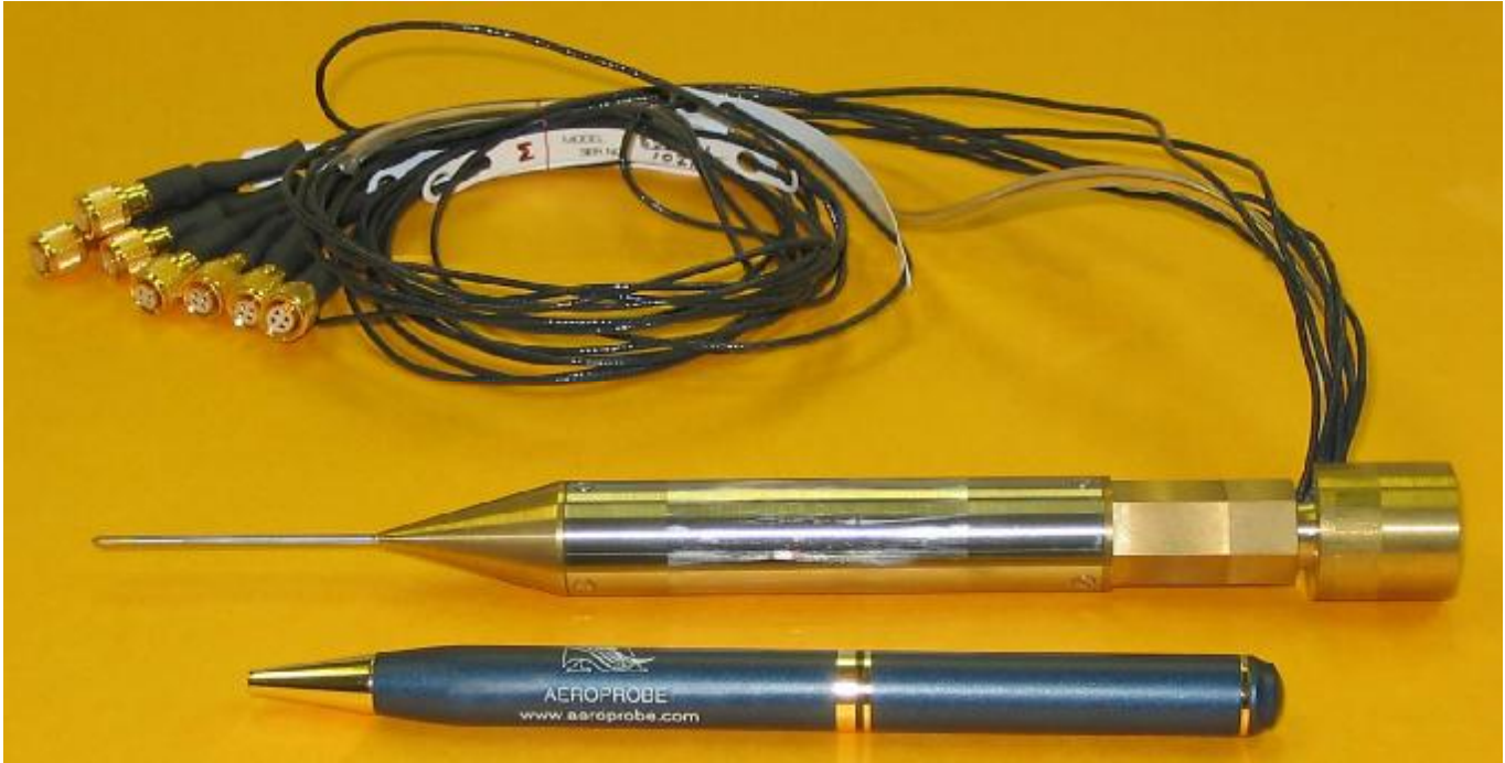
Aeroprobe Fast-Response Probe Model FRPS7-C160-152 (w/Calibration Mount)
