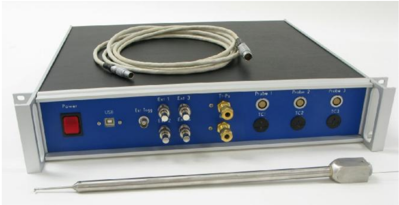
Fast-Response Aeroprobe, AMX4K Data Acquisition Module and Connecting Cable. Interface from Module to PC is USB Cable. Data Acquisition Driven by AeroAcquire, Integrating Multiprobe and ARC Software Packages for Reduction of Time-Accurate Flow Data.
