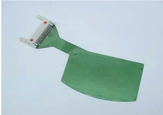
An Industrial TactArray Sensor (Brake-Pad Application)
