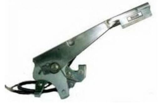
The ALF319 handbrake load cell offers an excellent technical solution to measurement of an ergonomic force. The double shear web design and rigid low profile finger grip combine to maintain the same precision of measurement along the entire finger grip length. The typical unevenly distributed force applied by the human hand is measured with good repeatability and minimum error in a sense normal to the lever axis.
