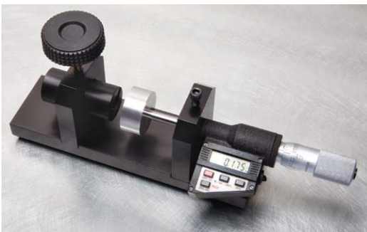
Calibration fixture 2U-16U sensors English/Metric 855578-001
