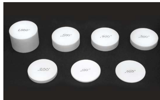
Calibration spacer set 26U-51U (0.050, 0.100, 0.200, 0.300, 0.400, 0.500, 1.000) 850859-001
