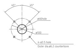
Note : 4 pcs. of mounting screws (M3 X8) are attached. (Unit : mm)
