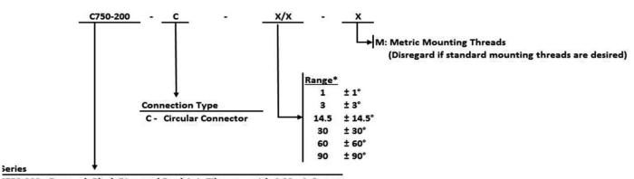
750-200 - Damped, Black Diamond Dual Axis Tiltmeter with 4-20mA Output
