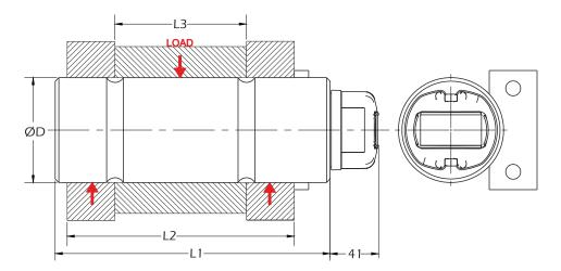
**Note:** Depending on the load pin diameter, it may be necessary to add a head of a larger diameter to accommodate the wireless housing. Generally this applies to pins with a diameter of less than Ø78mm.
