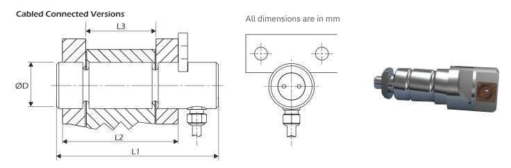
**Note:** Depending on the combination of pin diameter, cable type required and internal instrumentation, it may be necessary for the load pin to have a larger diameter head than the main pin diameter.
