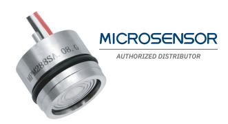
MPM288SA pressure sensor can convert pressure into standard electrical signal. It is composed of a PCBA circuit board with an ASIC chip and a standard  $\phi19\text{mm}$  piezoresistive pressure sensor. It can be flexibly assembled or welded to various pressure connections for different on-site pressure measurement instruments.
