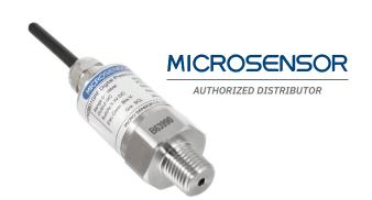
The MPM3801GRF digital pressure transmitter adopts the MPM3801 stainless steel oil-filled sensor as the sensing element, has the stainless-steel housing. Its wetted material is stainless steel, which has excellent corrosion resistance and long-term stability. The sensor is temperature compensated to ensure that the technical parameters such as zero point, sensitivity, linearity and stability are well maintained within the operating temperature range.
