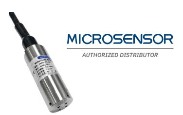
MPM4706 digital level transmitter is a highly precise and stable digital transmitter for the level measurement. This product utilizes the highly reliable piezoresistive OEM pressure sensing element and the high precision digital processing circuit, coupled with a dedicated algorithm, the transmitter is capable of high precision measurement.
