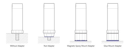
In case you would also like to measure the temperature of the machine, the optimal installation method is without an adapter. Only with this way the measurement point of the Industrial Node or Industrial Node 6 is deep enough below the machine surface to measure the temperature accurately. For detailed information about the different types of installation, please check the quickstart guide.
