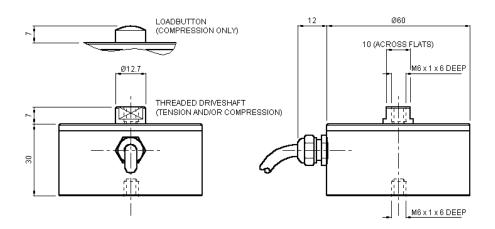
**Note:** The case height increases to 42 mm on the overload stop version
