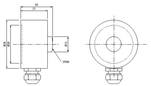
Dimensions in "mm", approx. values These drawings are for information only and not intended for construction purpose. Please contact us for detailed drawings.
