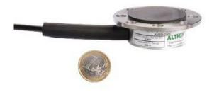
The ALF304 is a compact, low profile load cell for measuring brake pedal application forces. The load cell is robust in construction with a maximum force range of 2500 N (250 kg). Its multi-hole fixing allows simple attachment to any shape pedal using screws or cable ties. The low profile stainless steel design maintains the brake pedals ergonomic geometry.
