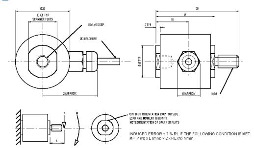
To optimise the performance the ALF308 end faces should be maintained parallel under load.
