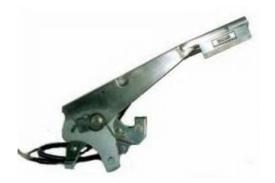
The ALF319 handbrake load cell offers an excellent technical solution to measurement of an ergonomic force. The double shear web design and rigid low profile finger grip combine to maintain the same precision of measurement along the entire finger grip length. The typical unevenly distributed force applied by the human hand is measured with good repeatability and minimum error in a sense normal to the lever axis.
