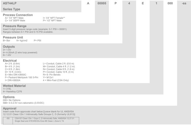
Note: CSA approved products require case/earth ground electrical connection. See wiring installation sheet for further details
