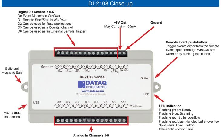
Voltage Range: ±10 Volts; Up to ±100V without damage
