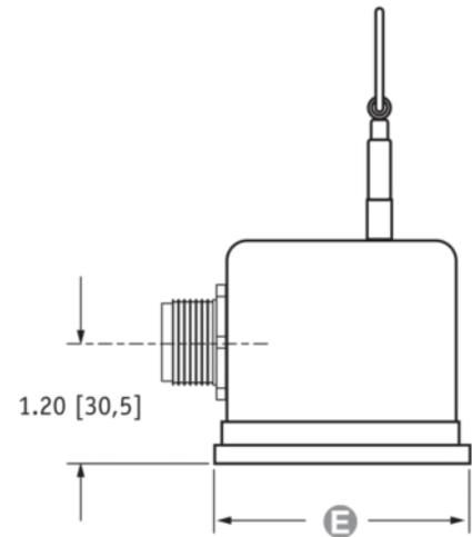
ALL DIMENSIONS ARE IN INCHES [MM] • tolerances are  $\pm 0.02$  in. [ $\pm 0,5$ mm]
