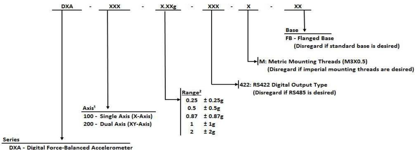
Example: DXA-100-0.25g = DXA series, single axis, ±0.25g range, RS485 output, imperial mounting threads, standard base
