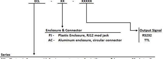
ECL - Electronic Compass with 3-axis magnetometer, 2-axis tilt sensor & low power 50 μA standby
