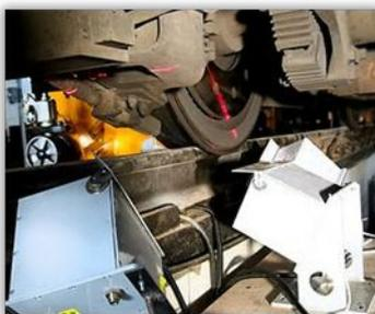
**Automatic real-time system for measurement of wheelsets geometrical parameters**
