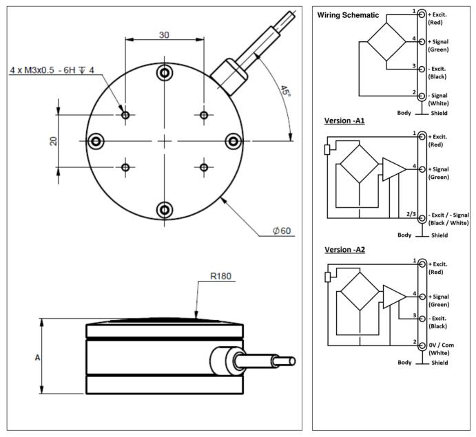
**Dimension A :** 28 mm for ranges 200N, 500N 29 mm for ranges 1kN, 1.5kN, 2kN, 2.5kN
