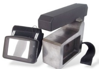
Railway Wheel Profile Gauge
