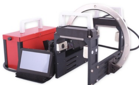
Rail Profile Measurement Gauge
