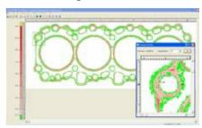
The specified field is enlarged. (×4,×8,×16) Pin point pressure values can be displayed on the image.
