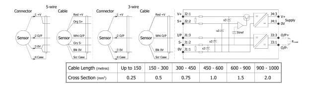
The table above shows recommended conductor sizes with respect to cable length for both three and five wire connections, based on copper conductors. Three wire connections will introduce a gain reduction of 5% and a  $\pm 1\%$  temperature dependence of gain over the range -40°C to +80°C for the cable temperature. (i.e. about -150 ppm/°C for the maximum lengths shown and less pro rata for shorter lengths.)
