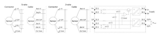
N.b. sensors supplied with cable, the free end must be appropriately terminated.
