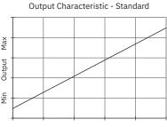
Retracted Linear Displacement Extended
