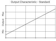
Retracted Linear Displacement Extended
