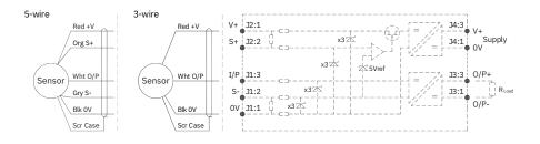
N.b. the free end of the cable must be appropriately terminated. Where the free end is to be terminated in a submerged position adequate sealing must be provided to protect connections.
