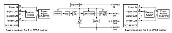
A through E: Connector pin assignments
