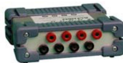
Passive modular enclosure for the conversion of up to 4 measuring signals 0(4) ... 20 mA into a precise 0(1) ... 5 V signal, e. g. for acquisition a GL820 or GL800 type datalogger.
