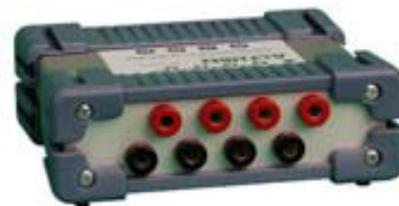
Passive modular enclosure for the conversion of up to 4 measuring signals 0(4) ... 20 mA into a precise 0(1) ... 5 V signal, e. g. for acquisition with a GL220 type datalogger.
