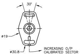
SHAFT FLAT ALIGNED WITH REFERENCE MARK IN BASE AT MID TRAVEL ±5°
