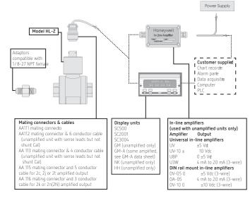
NOTE: For long cable runs or electronically noisy environments, an amplified sensor or locally mounted amplifier is often preferred.
