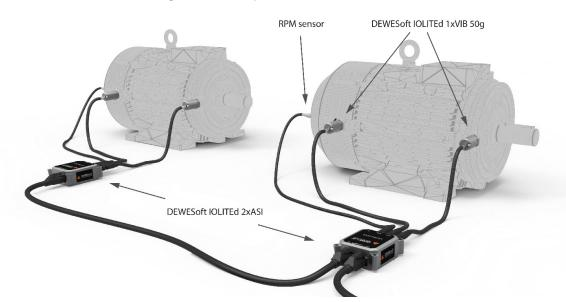
Microprocessor inside the DAQ module transmits the data samples over EtherCAT protocol into DEWESoft software running on a Windows PC, or alternatively to any controller running EtherCAT master on any platform.
