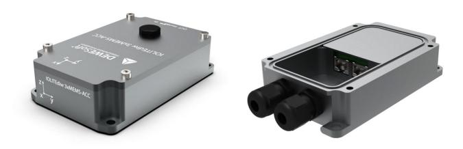
The outdoor enclosure automatically vents air to equalize pressure inside the enclosure to the outside air pressure while it does not allow water to pass into the enclosure. This prolongs the life span of the seal and increases durability of the enclosure.
