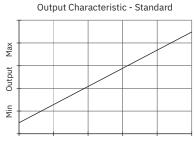
Retracted Linear Displacement Extended
