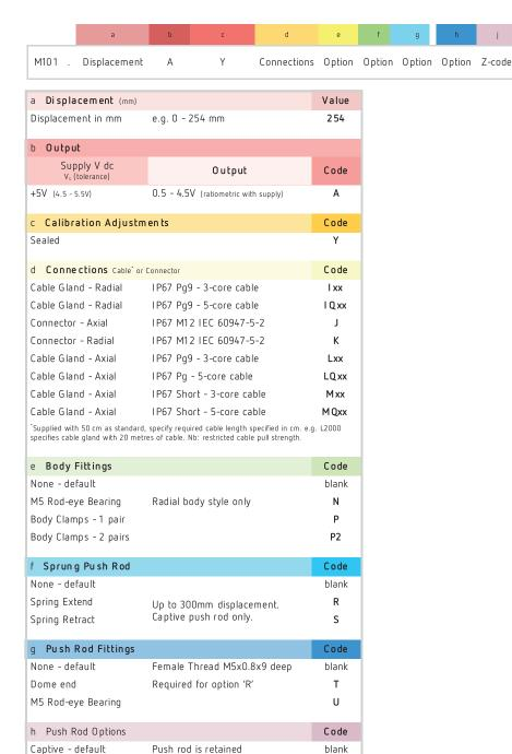
Note! All Intrinsically Safe (IS) sensors must have a Z-code suffix.
