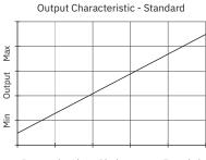
Retracted Linear Displacement Extended
