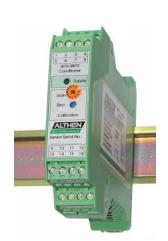
The LVDT measuring amplifier MC-KP for DIN top-hat-rail mounting offers supply and signal evaluation for LVDT transducers and gage head transmitters with an oscillator frequency between 1 kHz and 20 kHz. By use of multiple LVDT measuring amplifiers an oscillator voltage synchronization is possible. For further evaluation standard analogue outputs are available.
