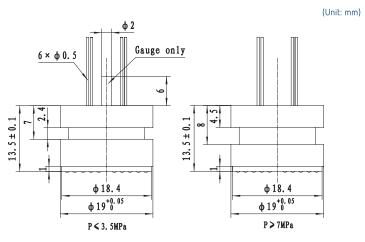
The suggested installation dimension is  $\Phi 19\,^{+0.05}_{+0.02}\,\text{mm}$
