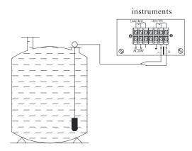
When measure static pressure in open tank, please put transmitter into tank bottom, and fix transmitter cable and connection box at the entrance of the tank.
