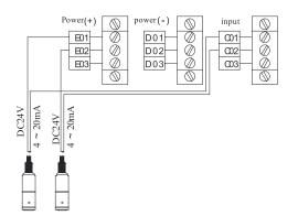
Connecting the most two level transmitter with MSB9438 measure displayer to build up one level difference system with multi-channel display. Output signal can be 4mA~20mA analog, it can also provide upper and lower limit control and alarm.
