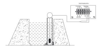
When measuring level in flow water, please insert one steel tube  $\Phi$ 45, and make some little holes $\Phi$ 5 at the different height of the tube. Make holes opposite to water flowing direction, and let water go into tube unobstructed. Fix cable and connection box at the entrance of the tube. OUTLINE CONSTRUCTION (Unit: mm)
