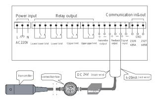
Connect Ex-proof version transmitter with safe barrier and measure displayer to build up one control system.
