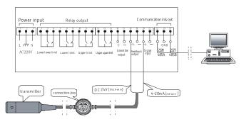
Connecting level transmitter with MSB9418 measure displayer to build up one level measure system with upper and lower limits control and alarming. Output signal is RS232 or analog 1 V~5V DC, 0V~5V DC, 4mA~20mA DC.
