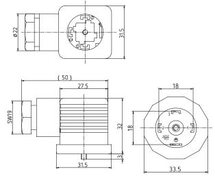
Applicable cable: 5-core with shielded sleeve OD: ø4.9 mm
