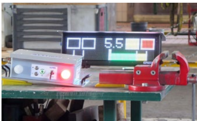
The remote LED display allows flexible, independent positioning of sensor and display.
