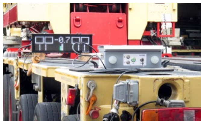
Perfect for heavy transport: The large LED display with automatic brightness control is easy to recognise at a distance of up to 20m.
