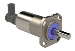
The P510 Rotary Inductive Position Sensor is an affordable, durable, high-accuracy rotary sensor designed for industrial and scientific feedback applications where the rotating shaft could be subjected to both axial and radial loading. The P510, like all Positek® sensors, is supplied with the output calibrated to the exact angle required by the customer, between 11 and 160 degrees.
