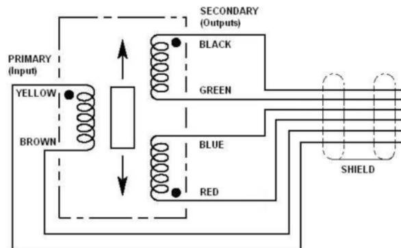
Connect Blue and Green wires together for differential output
