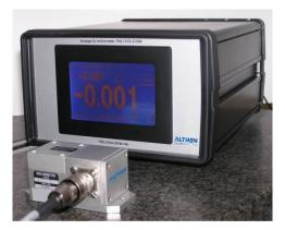
Microprocessor controlled single or dual channel readout with supply and signal conditioning for one or two inclinometers of type AILSO with ranges from  $\pm 1^{\circ}$  to  $\pm 90^{\circ}$ .
