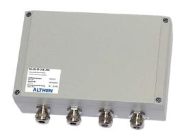
The dual-channel strain gauge measuring amplifier SG-2K-IP allows supply and signal evaluation of two connected transducers with a strain gauge full bridge greater than 300 ohms. Input and output are galvanically isolated. The connection is done in 4-wire technology. For further evaluation standard analogue outputs are available. The measuring amplifier is built-in into a robust EMC die-cast aluminium enclosure (IP65) which is suited for application in rough and industrial environments.
