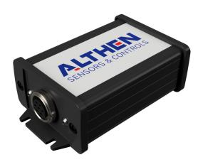
The SG-INL2 1-channel inline strain gauge measuring amplifier in a robust aluminium housing (IP54) enables the power supply and signal amplification of a strain gauge transducer. Any strain gauge transducer with a strain gauge full bridge resistance greater than 300 ohms can be connected. The transducer is wired using 4-wire technology.
