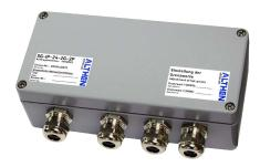
The single-channel strain gauge measuring amplifier SG-IP-2G-2P allows supply and signal evaluation of two parallel connected strain gauge transducers with standardized sensitivity. The connection is done in 4-wire technology. For further evaluation standard analogue outputs are available. A test signal and 2 threshold value set-points as well as potential-free switching contacts (max. 30 VDC/0.5 A) for limit value monitoring are available for further evaluation.
