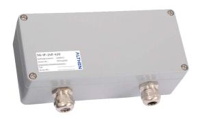
The single-channel strain gauge measuring amplifier SG-IP allows supply and signal evaluation of one transducer with a strain gauge full bridge greater than 300 ohms. Input and output are galvanically isolated. The connection is done in 4-wire technology. For further evaluation standard analogue outputs are available. The measuring amplifier is built-in into a robust EMC die-cast aluminium enclosure (IP65) which is suited for applications in rough and industrial environments.
